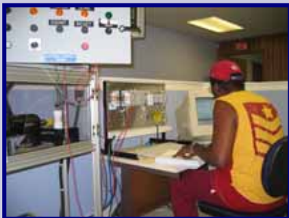
Student working through a lab assignment using AB MicroLogix1500 PLC hardware and AB RSLogix500 software.
