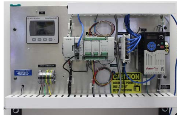
Hale Automation Trainer with Allen-Bradley Micro850™ Programmable Controller.
