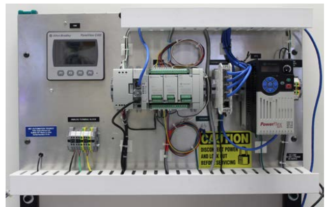
Hale Automation Trainer with Allen-Bradley Micro850™ Programmable Controller. Rockwell Automation's Connected Components Workbench (CCW) programming software is available free of charge from www.rockwellautomation.com
